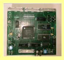
**9.13.** Set up of a **Z86C95 DSP development kit** (a complet technology, hard and soft: development board, monitor, crossassambler, C compilator), for Z86C95 microcomputer with Digital Signal Processor -1996, ITC. The C compilator was written by Laura Galiş)
