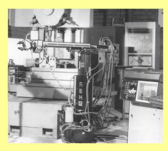
**9.5.** Commmand unit for a hydraulic-mechanical industrial robot - REH-02\*, (with Polytechnical University of Cluj-Napoca), 1983/1984,
