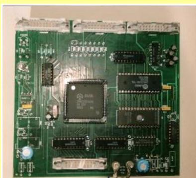
**9.13. Set up of a Z86C95 DSP development kit** (a complet technology, hard and soft: development board, monitor, crossassembler, C compiler), for Z86C95 microcomputer with Digital Signal Processor -1996, ITC. The C compiler was written by Laura Galis)
