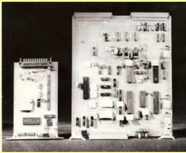
**9.8. Technological development** in 1986/87: swept from  $\mu$ processor (Intel 8080) to one chip  $\mu$ controllers (Z8), for industrial applications (Robots Command Units – see <http://www.itc-cluj.ro/CelulaRobot.pdf>)
