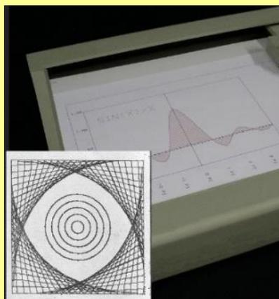
**9.4. MD-10 - first Romanian Plotter**, - 1979/81 designed for mass production at IEPER (Company for computer peripheries equipment) Bucharest.
