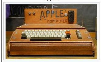
A fully assembled Apple I computer with a homemade wooden computer case
